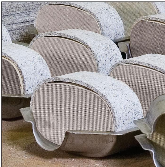
Ceramic substrates are coated with a washcoat containing precious metal catalysts prior to installation into the converter can.
