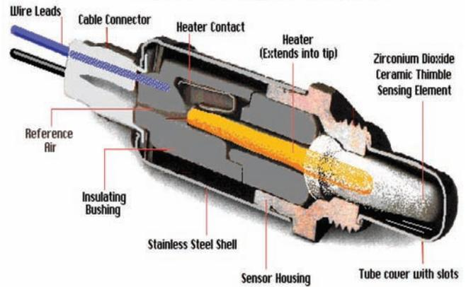
**QUESTION: I would like to know, what's the difference between a “heated” and “unheated” oxygen sensor?**
