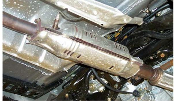
Conversely, a really good converter should clean the exhaust so well that it almost puts the rear sensor to sleep, or flatline at .20 volt. But the PCM has to know the rear sensor is working, so it attempts to drive it to the middle of its range.
